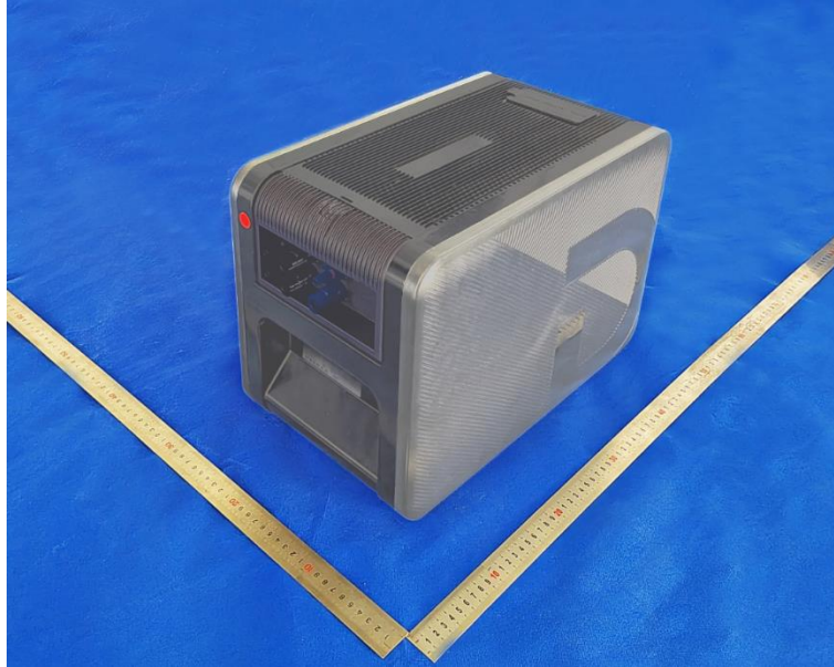
Photo 1 电池组正面 Front view of battery
